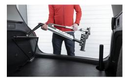
The clever design of the Carolift 100 shines through in its ease of use. Open your boot, deploy the lift over your mobility device and lower the lift arm. Once within reach, you connect the clever lifting straps. Use as much slack as you need to fit the buckle on the mobility device. Pulling on the loop will tighten both sides simultaneously. Don't worry if the strap is longer on one side. The Carolift 100 will self-balance the load as soon as it leaves the ground.
