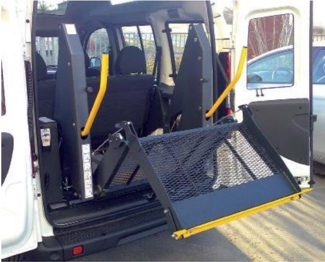
The Toyota Commuter is a large sized van with versatile configurations available. This type of van can be paired with a rear platform lift to fit the size of most larger powerchairs.
