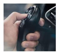
The **My Command** is an ergonomic steering device used to control not only the steering but all the auxiliary functions required to operate the vehicle. With up to 14 functions available, you can tailor the functions to suit your driving needs.
