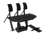
The **Stamp Pedal Extension** enables an extension of 10-30 cm. Adjustments can be made for distance, height and the desired space between pedals. They are also fitted with a quick release, to be easily removed.
